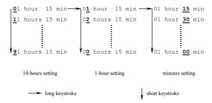
Activate the countdown timer by leaving the timer setup menu with a long keystroke. Alternatively, the countdown is started automatically if you do not change any setting for longer than 12 seconds.
