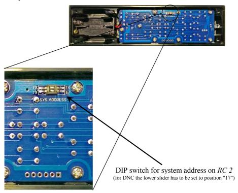
To configure the Audionet Metal Remote Control *RC 2* for controlling the DNC, put the lower slider of the DIP switch labelled 'SYS AD-DRESS' in position "17".
