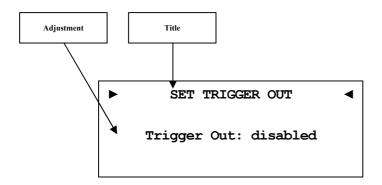
Use trigger output **TRIGGER** 7 to control (e.g. switch on/off) non Audionet devices. If you switch on the DNC from stand-by mode, the trigger output 7 provides a signal of 12 Volts DC.
