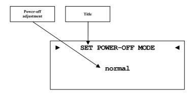
There are two different power-off modes available for the DNC. Firstly the **normal** power-off mode and secondly the **Quick Start** mode.
