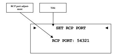
Enter the port number for communication between DNC and the software Audionet RCP or Android app aMM or iOS app iMM. If necessary, you may adjust the port number in a range of 50000 to 59999. The factory default value is 54321. Changing the default value will only be necessary if this port number is already used in your network. If necessary, ask your network administrator for support.
