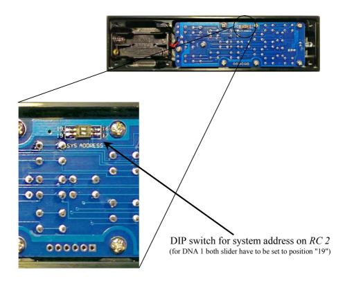
To configure the Audionet Metal Remote Control *RC 2* for controlling the DNA 1, put both sliders of the DIP switch labelled 'SYS ADDRESS' in position "19".
