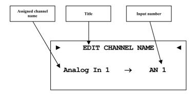
You can assign a fully user-definable name up to 12 characters in length to each of the thirteen input channels. The display shows the number of the currently selected input channel and the assigned channel name. The cursor marks the character you now may alter.
