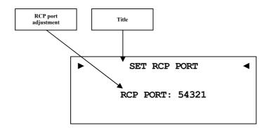
Enter the port number for communication between DNA 1 and the software Audionet RCP or Android app aMM or iOS app iMM. If necessary you may adjust the port number in a range of 50000 to 59999. The factory default value is 54321. Changing the default value will only be necessary if this port number is already used in your network. If necessary, ask your network administrator for support.
