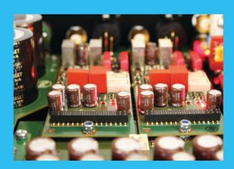
The Primary amplification is performed in the transistor input stage by our double mono construction, fitted with double FET inputs. With no error current, these provide unlimited input resistance, and under conditions of minimal constant capacity have an almost unlimited input resistance.
