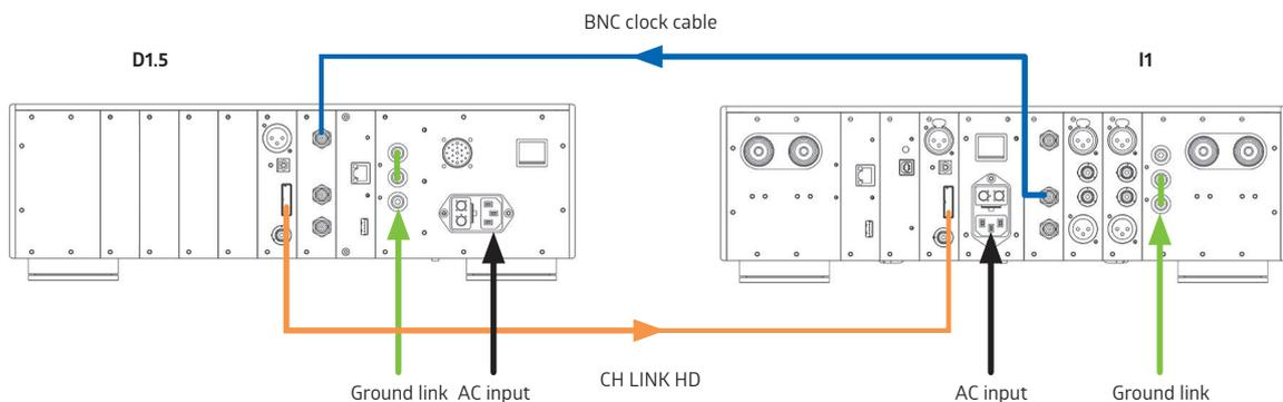
More generally, when a D1.5 has no SYNC\_IO board, it can only reference itself to its internal clock, and the DAC has to recover the clock signal from the audio data. In such cases you should configure clock settings as follows:
