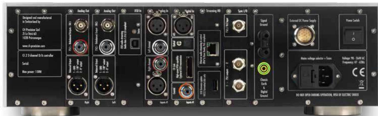
to configure the C1.2 specifically to their system and replay requirements. Alongside the multiple digital input and clock-sync options, there is also a by-passable hybrid volume control, operating across both the analog and digital domains and an A-to-D facility, allowing the C1.2 to accept balanced or single-ended analog inputs, creating a genuine analog/digital domain control option, allowing the C1.2 to stand at the center of any system, irrespective of the source components in use.
